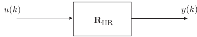
Figure A.6: A SISO system \mathbf{R}_{\text{IIR}} with input u(k) and output y(k) .
