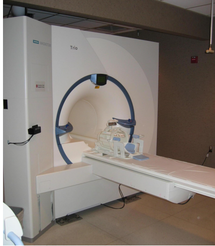
Figure 1.4: A photograph of an MRI scanner. The patient lies on the small table that slides into the scanner.
