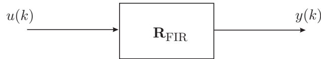
Figure A.2: A SISO system \mathbf{R}_{\text{FIR}} with input u(k) and output y(k) .
